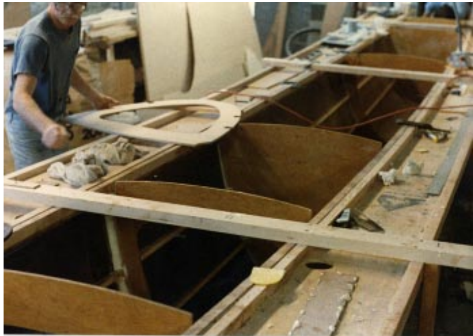
Installing bulkheads and stringers.
