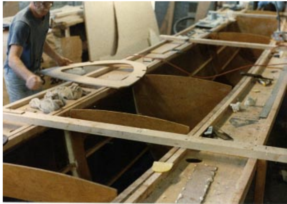
Installing bulkheads and stringers.
